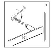
8. Install the Handle Set[6] onto the Door Panels[5&16], lock and fasten them with Allen Key. Please see Fig 1 for details.
