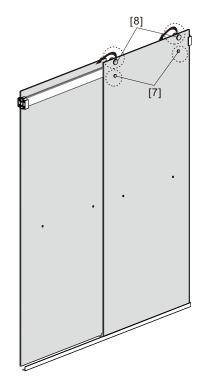
7. Install the Top Rollers[8] into the two predrilled holes of the Door Panel[16]. Place the bottom of Door Panel[16] into the gap between the Door Guide[10] and Bottom Horizontal Rail[13], and insert the top of Door Panel[16] into the slot of Top Horizontal Rail[8]. Install the Anti-collision Component[7] into the hole of Door Panel[16],lock and fasten it.
