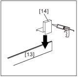
10. Apply thin beads of glass glue into the Cover Caps[14], and assemble them on both ends of the Bottom Horizontal Rail[13].
