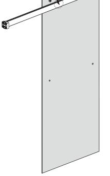
5.Install the Top Wheels[4] through the pre-drilled holes in Door Panel[5]. Stick the Top Wheels[4] in the openings of the Top Horizontal Rail[9].
