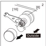
9. If there is a seam when the door is closed like the picture in the right, use Wrench to adjust the Top Wheel[4] or the Top Roller[8] till there is no seam any more.
